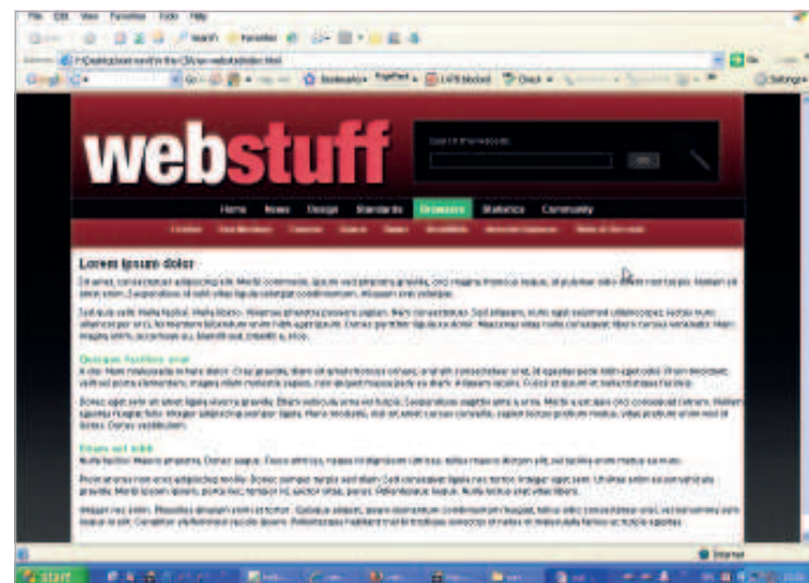
Without the hacks If you don't add the rule in the 'ie-hacks.css' style sheet, IE fails to draw some elements. The fix? Define a set height for specific elements in an IE-only style sheet
