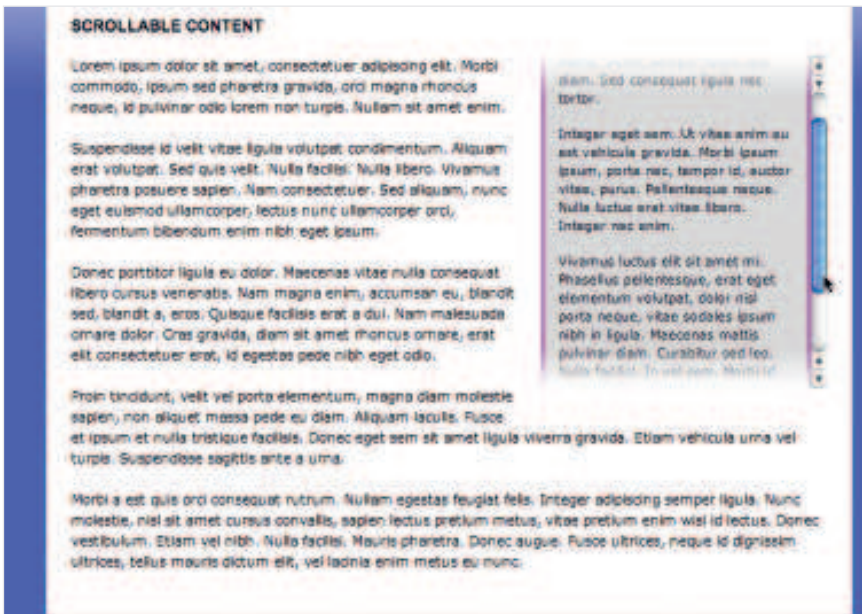
The final result This tutorial's web page, with its right-floated div offering scrollable content that fades into the background, thanks to two cunningly positioned divs with PNGs
